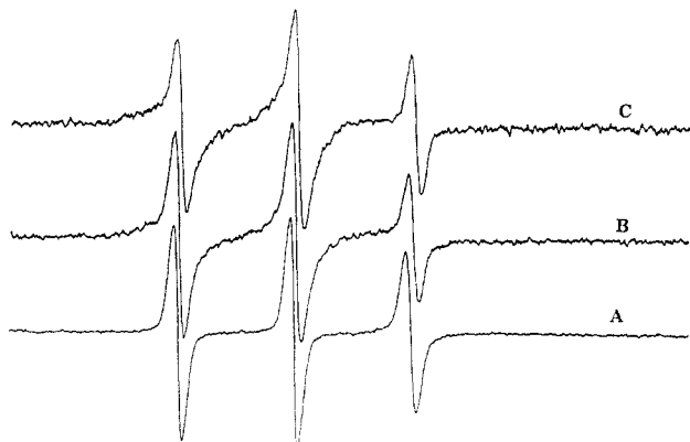
Figure 8. ESR spectra for 0.45% \kappa -carrageenan/0.15% konjac mannan mixture in 50 mM KCl illustrating the onset of line broadening close to the temperature corresponding to peak I in the DSC cooling curves: (A) above the gelation point; (B) at the gelation point; (C) below the gelation point.
